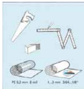
Fig 4. Required for installation • pencil • saw • spacers • measuring tape • 2mm closed cell moisture barrier underlay
