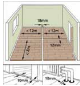
Fig 14. Architraves (doorways) can be installed with a 10mm expansion gap. Alternatively, the architrave can be undercut a little higher than the thickness of the board. Adequate expansion must still be left.
