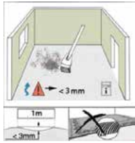
Fig 1. Ensure that the subfloor is clean and level. Using a 1m straightedge, the subfloor level should not exceed 3mm over 1 lineal metre in any direction. Uneven subfloors will effect the performance of the product and may lead to product failure and can cause noise. Floors can be levelled with a self leveling compound and high spots can be grounded/sanded. The product can be installed over well adhered and level vinyl, cork, ceramic tiles and timber floorcoverings (never over other floating floorcoverings) The product cannot be installed over carpet and or carpet underlay.
