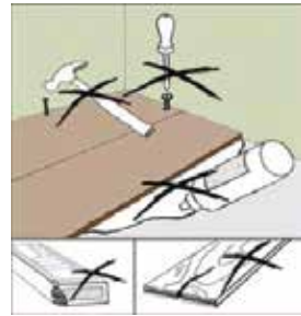
Fig 3. The product is recommend to be installed as a floating floor. It is not recommend to nail, screw or adhere product to the sub floor with adhesive.
